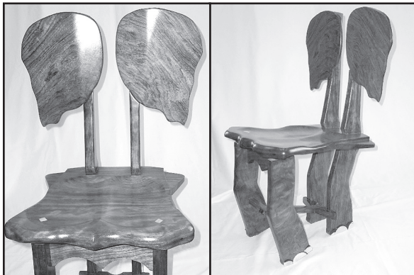
Elephant chair made for my grandson. Wood is Bubinga, with Ebony and Tagua Nut inlays for the toe nails.
